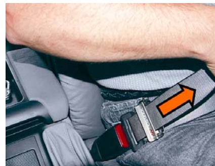
8. Buckle up as usual, then simply pull the slack out of the lap belt by pulling the shoulder belt as shown by the red arrow. If you need more slack to buckle up, depress the lever to let the seatbelt slide through the CG-Lock.
